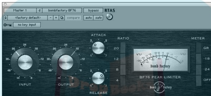
Figure 4-3: The Bombfactory BF76 peak limiter plug-in limits the maximum level of the signal passing through it.
